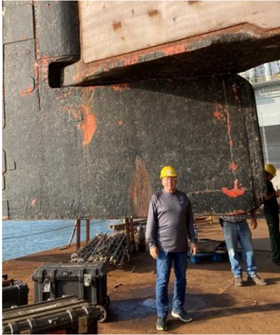
Figure 3. The author, standing next to the battleship's rudder. The rudder is turned 14° to starboard. It has been stuck at this angle since 1948. Photograph by John Nuckols.
